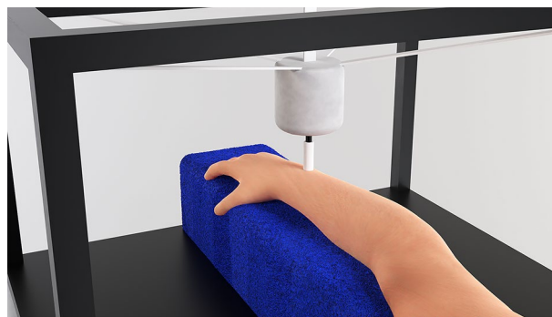
Figure 7. 3D render of the EHS Research Group haptic stimulation rig, shown from the participant's point of view, with the arm resting on a blue foam surface and the probe (attached to the shaker unit) contacting the centre of the dorsal wrist.
