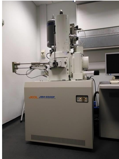
Figure 3.4 Scanning Electron Microscope (SEM, JEOL – JSM6500F)
