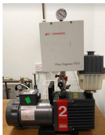
Figure 3.5 Plate degasser, Edwards PD3
