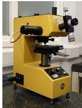
Figure 3.3 Vickers hardness indenter (Matsuzawa)
