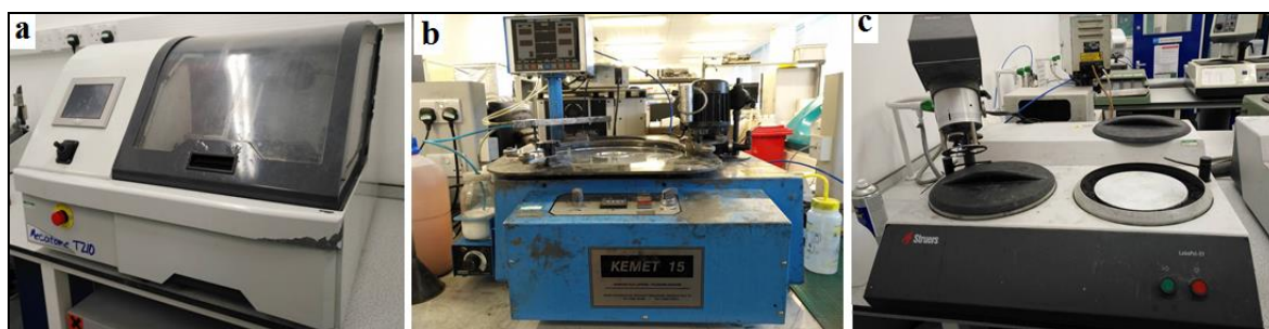
Figure 3.2 (a) Precision saw, (b) Lapping machine, (c) Polishing plate
