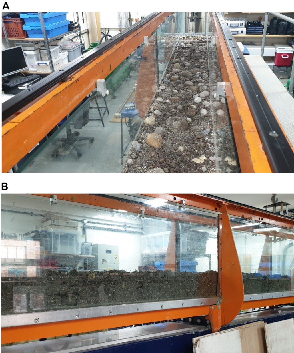
Figure 5.3: The artificial chalk stream gravel bed set-up in the experiments from (A) above and (B) the side of the flume.
