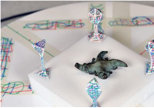
Thomas Allison's 3D printed capture targets for the gold weights at Pitt Rivers Museum
