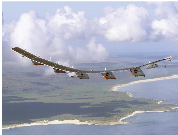
FIGURE 2.12: Helios in flight [111]. This UAV has a wingspan of 75 m and a gross mass of up to 929 kg.
