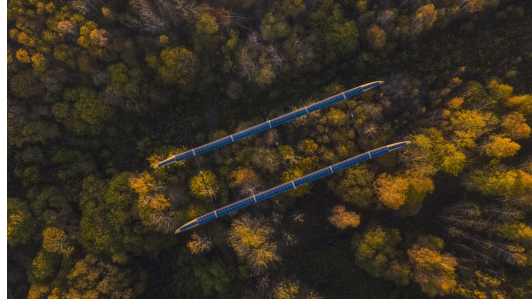
FIGURE 2.10: APUS DUO 15 [153]. The aircraft has a wingspan of 15 m and a gross take-off mass of 43 kg.
