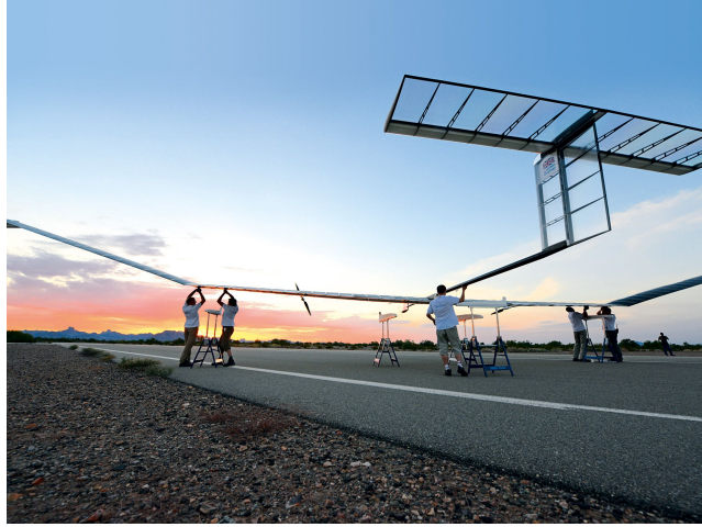
FIGURE 2.11: High Altitude Pseudo-Satellite (HAPS) Zephyr in preparation before take-off [5]. This UAV has a wingspan of 25 m and weighs less than 75 kg.
