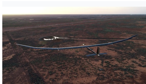
FIGURE 2.8: PHASA-35 [15]. The aircraft has a wingspan of 35 m and a gross take-off mass of approximately 150 kg.
