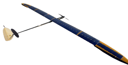
FIGURE 2.9: SAT i [153]. It has a wingspan of 7.3 m and MTOM of 6.3 kg.
