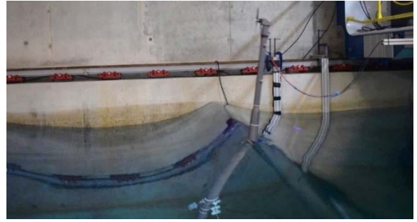
1380 1381 Figure 21: Effect of a rogue wave on a moored 1382 floating wind turbine model. A propeller is used to 1383 represent the wind turbine thrust. 1384
