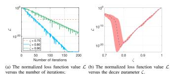
Fig. 5. The convergence behavior of the proposed gradient descent algorithm for optimizing a SIM to fit a 2D DFT matrix with (2,2) grid points.
