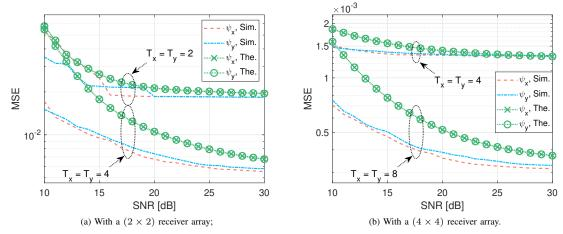
Fig. 9. The MSE of the SIM-based DOA estimator versus the effective SNR, where the abbreviations 'Sim.' and 'The.' refer to the simulation results and theoretical analysis, respectively.
