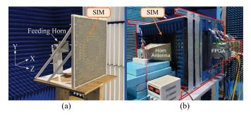
Fig. 1. The photographs of the existing SIMs. (a) A three-layer SIM in ©IEEE [27]; (b) A five-layer SIM in ©Nature [25].
