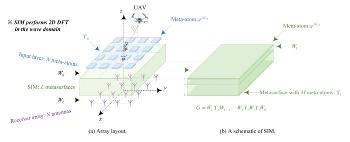
Fig. 2. A SIM-aided array system.
