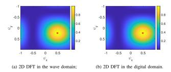
Fig. 7. Angular spectrum of the incoming signal using a  $(2 \times 2)$  receiver array, where we have  $\bar{\psi}_x = 0.48$  and  $\bar{\psi}_y = 0.23$ . The red cross represents the true DOA position on the spectrum.
