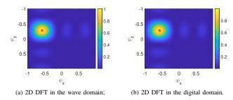
Fig. 8. Angular spectrum of the incoming signal using a  $(4 \times 4)$  receiver array, where we have  $\bar{\psi}_x = -0.58$  and  $\bar{\psi}_y = -0.28$ . The red cross represents the true DOA position on the spectrum.
