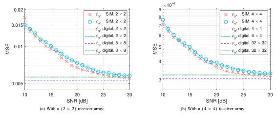
Fig. 10. Performance comparison of the SIM-based DOA estimator and the conventional approach via a 2D digital DFT.
