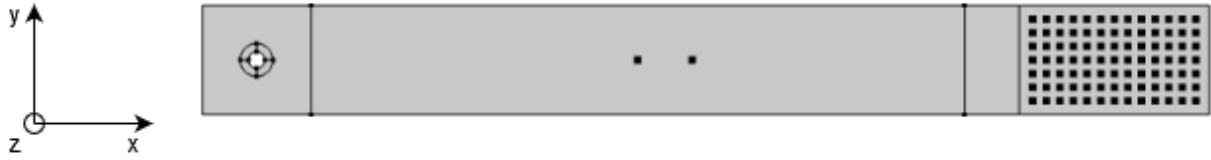
Figure 1: Numerical model viewed with the z -axis out of the page, showing the grid of points in the ABH taper section used in the stress calculation on the right hand side.
