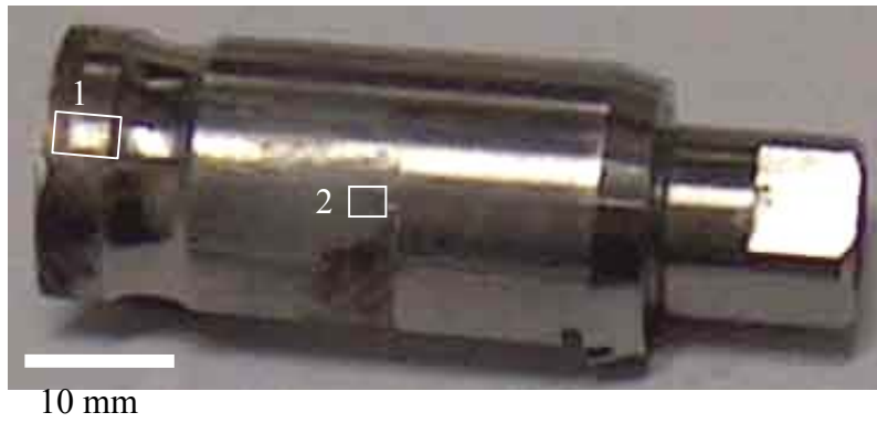
Fig. 1: A photograph of a failed insert after service.
