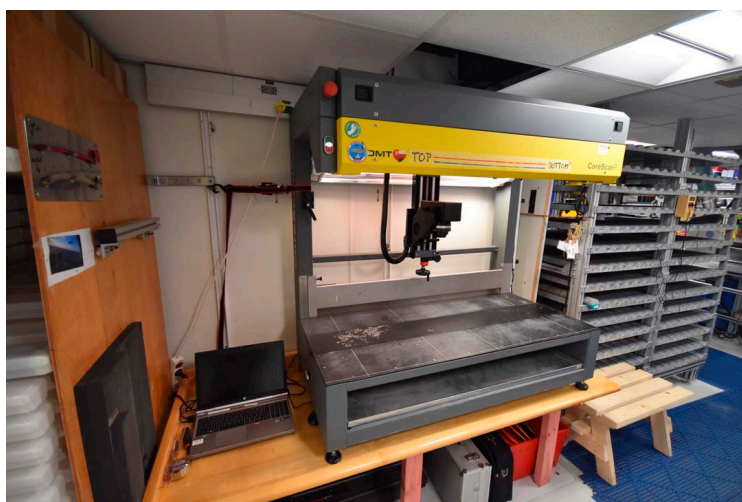
Figure F1. DMT CoreScan3 system used aboard JOIDES Resolution , Expeditions 390 and 393.
