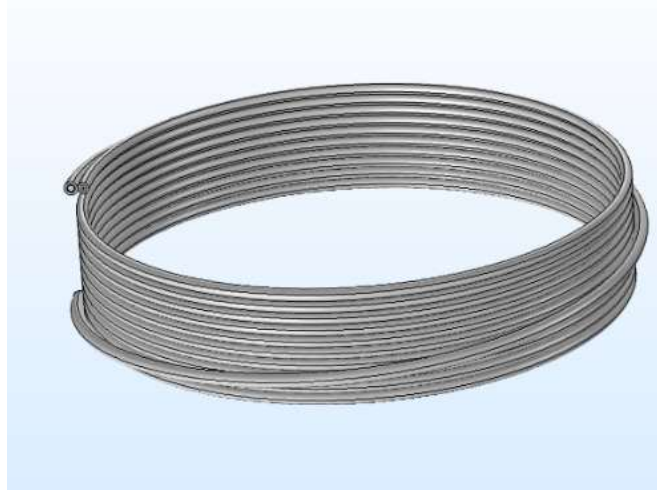
FIGURE 4.4: 3D module of fibre coil composed of HCF and SMF (built in COMSOL)
