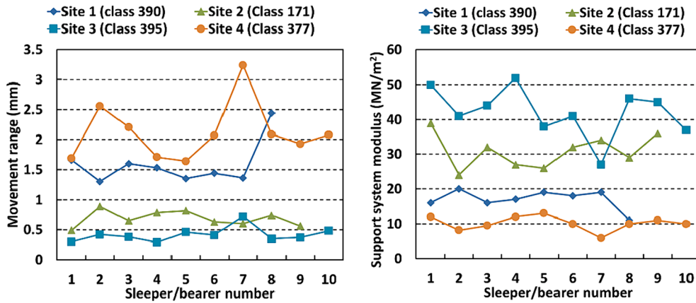
Fig. 2. (a) Measured deflections and (b) inferred rail support system stiffnesses on well-performing track (Powrie, [36]).
