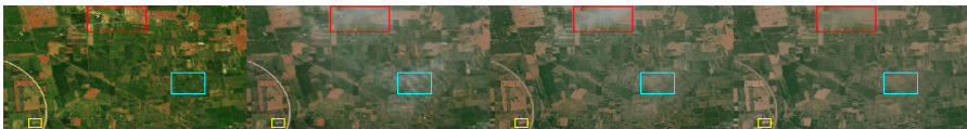
Fig. 5 The RGB image of a scene. From left to right, the images are: the ground truth (the cloudless reference image), the cloudy data image \mathbf{M} , the reconstruction obtained by FroNMF on \mathbf{M} , and the reconstruction obtained by Chordal-NMF on \mathbf{M} . In the image, the three color-boxes are selected areas under different cloudiness in which we perform further quantitative analysis.
