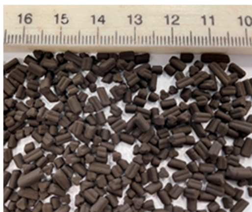
Fig. 4. Image of the C-based oxygen carrier (OC) used in this experimental study.
