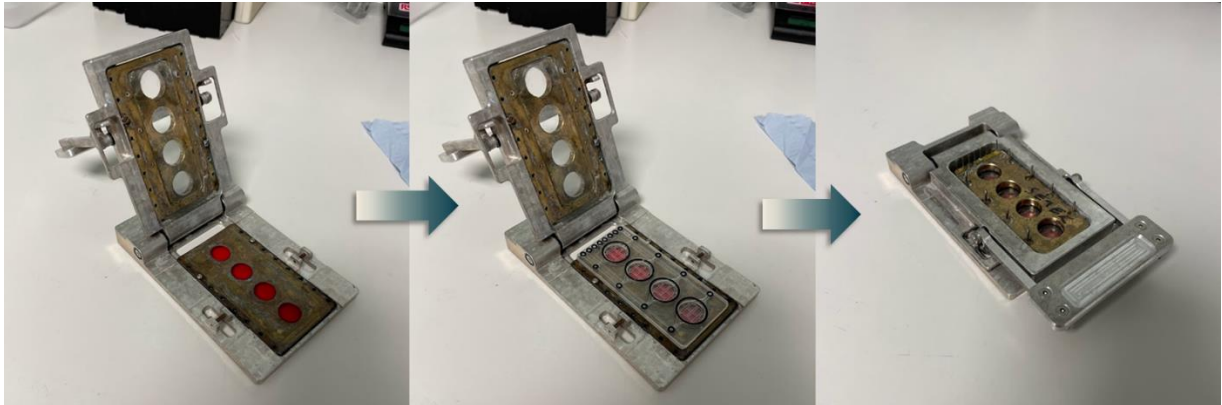
Figure 3.50: Setting up the system. First, the chip holders are clean and the filters place in the holes. Next, the device is aligned in the bottom holder and the O-rings places in their grooves. Finally, the chip holder is closed by the clamp, sealing the four chambers simultaneously.
