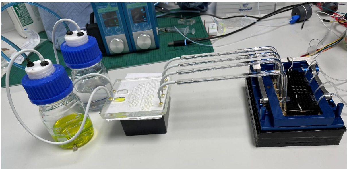
Figure 3.36: New setup with the serial dilutor as the gradient generator and the multichamber device (Device v3) mounted on the chip holder and on the electronic oxygen detector.
