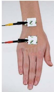
Figure 5. Placement of electrodes on hand
