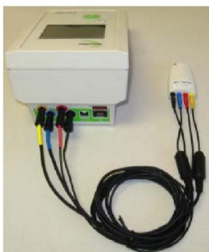
Figure 11. The leads connected to the calibration Test Cell
