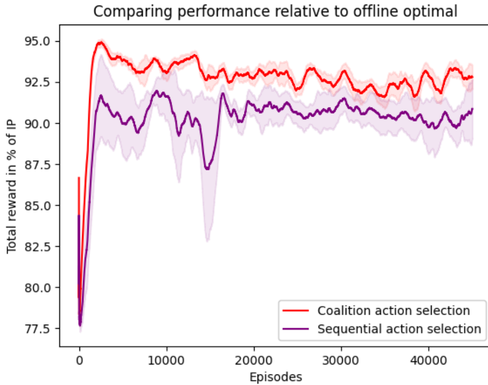
FIGURE 4.4: Convergence of the stationary ASO input transformation-based DRL algorithm on the coalition action selection and the sequential action selection using step-by-step training
