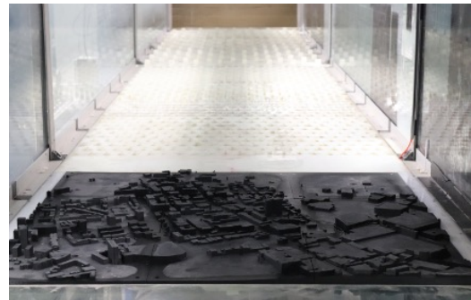
Figure 2. An image of the experimental setup used in this experiment series. In this image the upstream roughness elements are visible, followed by the 3D printed city model.
