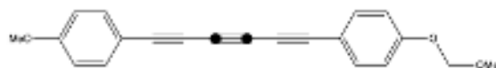
FIG. 1. Schematic representation of I , with black circles representing ^{13}\text{C} labels. The different substituents at the ends of the molecule give a small chemical shift difference of 0.16 ppm between the two ^{13}\text{C} sites.
