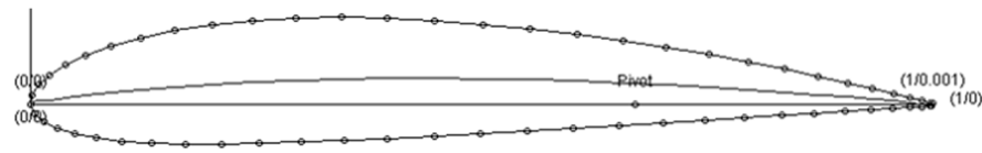
Figure 4. NACA3414 airfoil profile (JavaFoil, 2024) [27].
