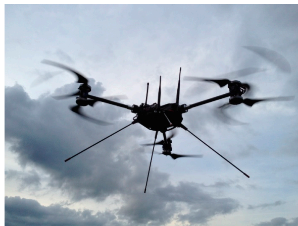
Figure 2. Example of a small Y6 drone (HALO), winner of the DARPA UAVForge challenge 2012.
