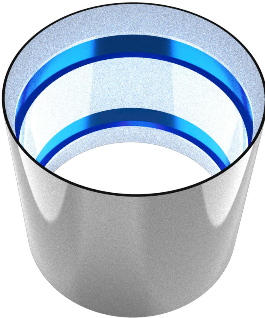
Fig. 2. Concept model of the holding member design for e-TAVI. The magnetic regions are coloured in blue for emphasis, facing radially inward. The exchangeable valve would be deployed within the holding member and the ferromagnetic regions on the frame would be attracted to these magnetic regions. This image is purely conceptual; in reality the member would need a suture ring for surgical implantation or a crimpable frame holding the magnetic regions for delivery via catheter. (For interpretation of the references to colour in this figure legend, the reader is referred to the web version of this article.)
