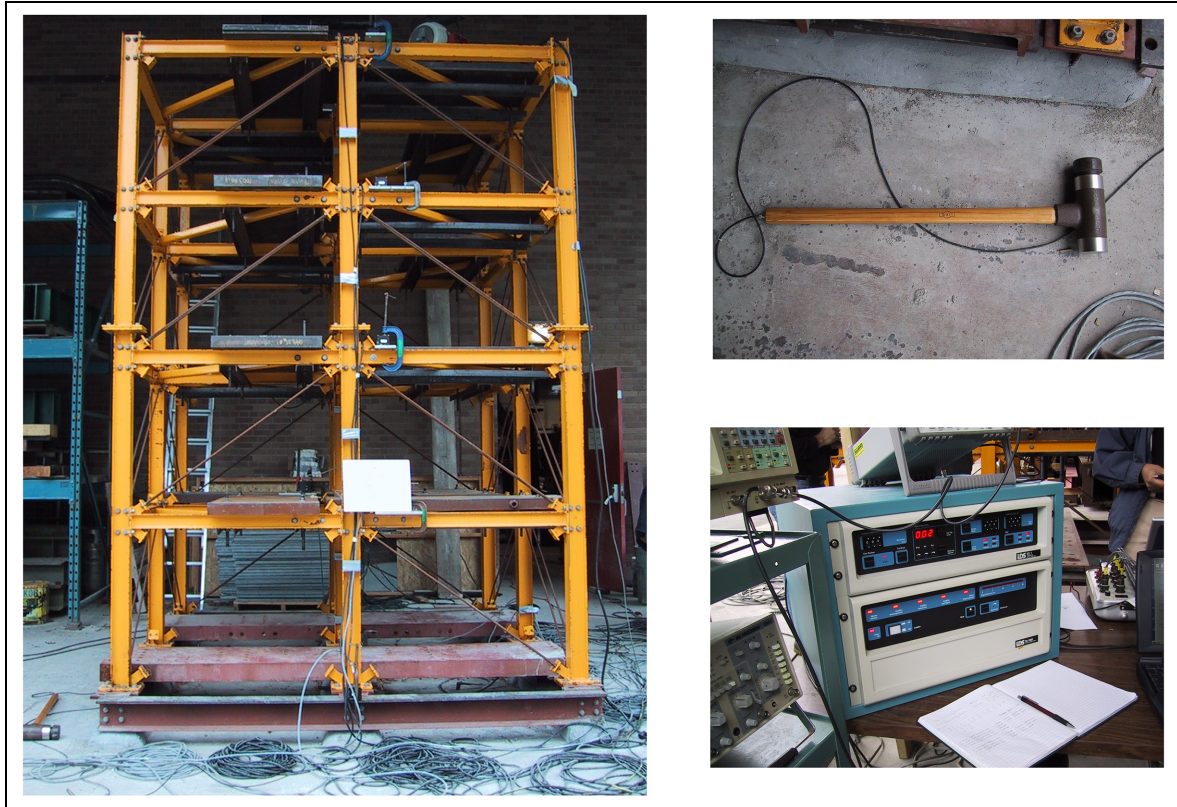
Figure 12. IASC-ASCE structural health monitoring benchmark building of section “Structural loading identification in the IASC-ASCE structural health monitoring benchmark problem”, the Dynatron 5803A 12 lbf Impulse Hammer, and the monitor and console equipment. 115
