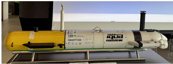
Fig. 3: The “Smarty200” Iqua Sparus II AUV owned and operated by the University of Southampton. The AUV is modified to integrate a high-resolution seafloor imaging system and a Doppler aided inertial navigation system.
