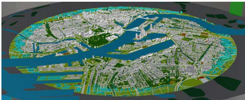
Figure 1: Visualisation of the 3D CFD model of the inner city of Rotterdam
