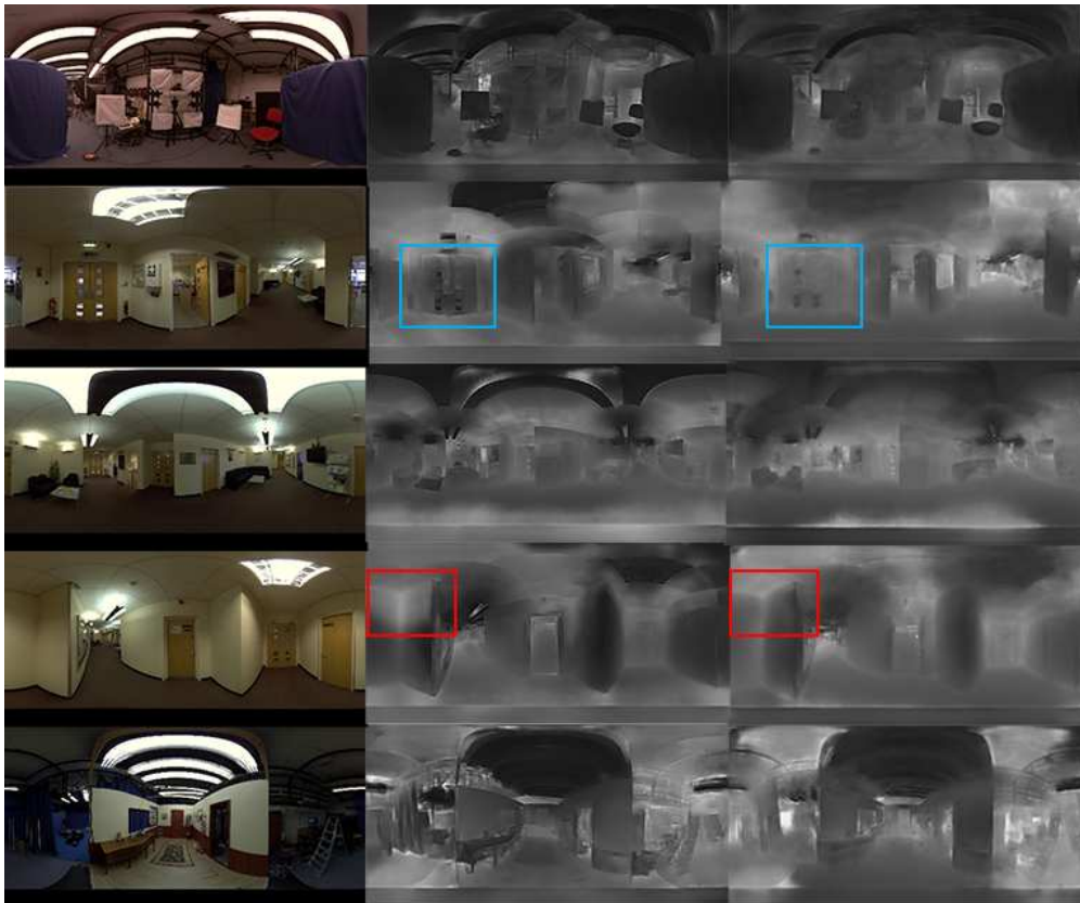
FIGURE 4.6: Performance on a New Real-world Dataset (left: RGB images of scenes, middle: AdaBins, right: proposed architecture)
