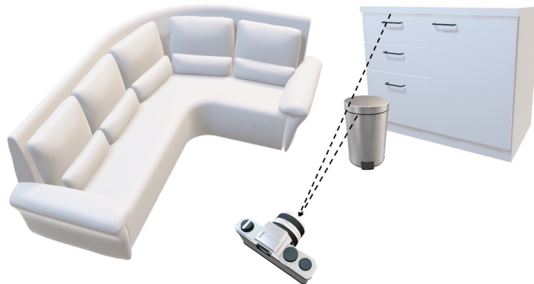
FIGURE 5.1: The Example Scene Showing How the Depth of an Object Changes along the Direction of Gravity.
