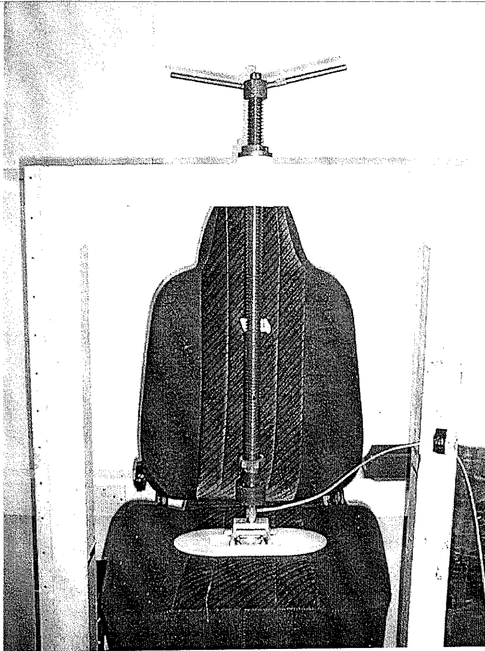
Figure 3 Use of load cell to measure force applied by the indenter (using SIT-BAR as indenter head).
