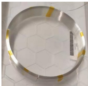
Figure 5.13 Photograph of the prepared support-free HCF coil (diameter of 160 mm; pitch of 500 \mu\text{m} ; N_{tot} = 19 ; 57 turns).
