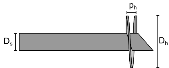
Figure 10. Sketch of a screw pile (rotated 90°). D_h and p_h are the helix diameter and pitch and D_s is the shaft diameter. widely used onshore, but their use offshore requires a significant upscaling in their dimensions and the
