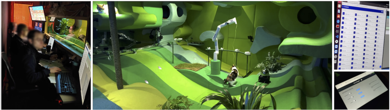
Figure 1: Left: The control room (front to back): robot operator, artists, vision mixer. Centre: Inside the Cat Royale enclosure, in the centre of the room is Clover playing with the String deployed by the Robot. In the upper left corner Pumpkin is resting on one of the high perches. Behind the robot are the four toy racks used to store end-effectors. Two of the high dens are visible, allowing the cats to retreat. On the left, a scratching post, as well as the ball run tube system is visible. Within the enclosure a multitude of plants are distributed. Right top: The robot control system. The activity library is on the left. Each blue box (52 visible) represents one of the many possible robot actions. Right bottom: The iPad based interface for documenting the cat stress score [28], this is based on a seven point scale (1: Fully Relaxed to 7: Terrified).
