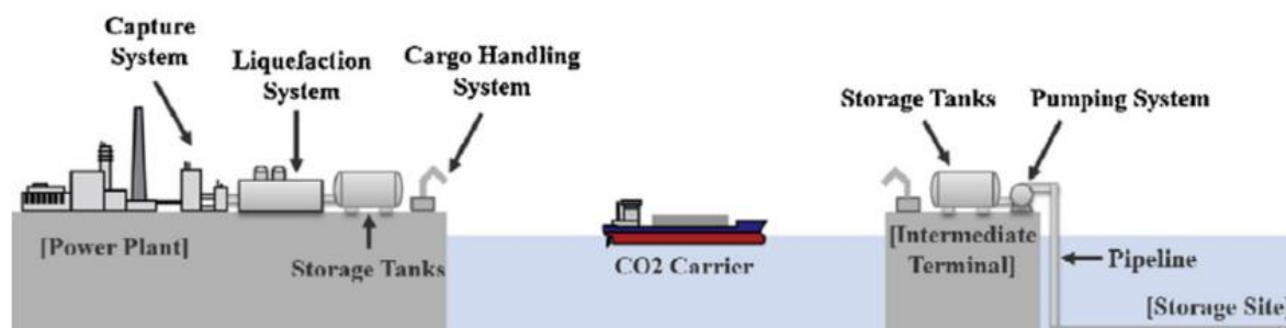
Figure 4. Components of the CO 2 capture, storage and shipping chain ([33], [34])
