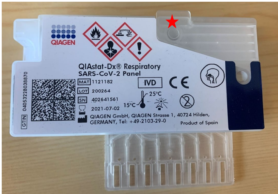
Figure 25: The QIAstat-Dx Respiratory panel test cartridge
