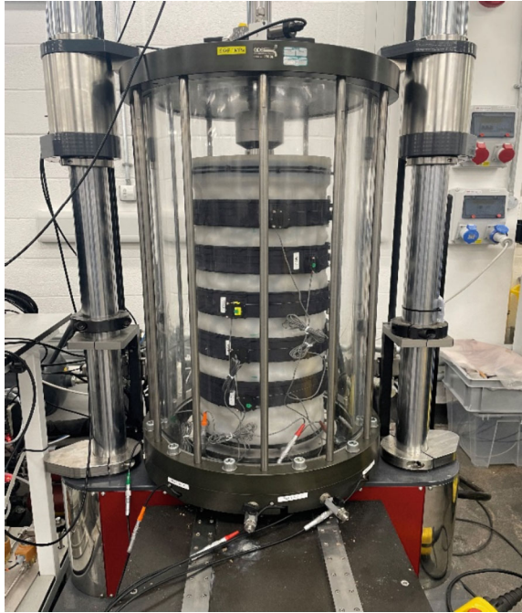
Fig. 1 Triaxial set-up with 5 radial belts
