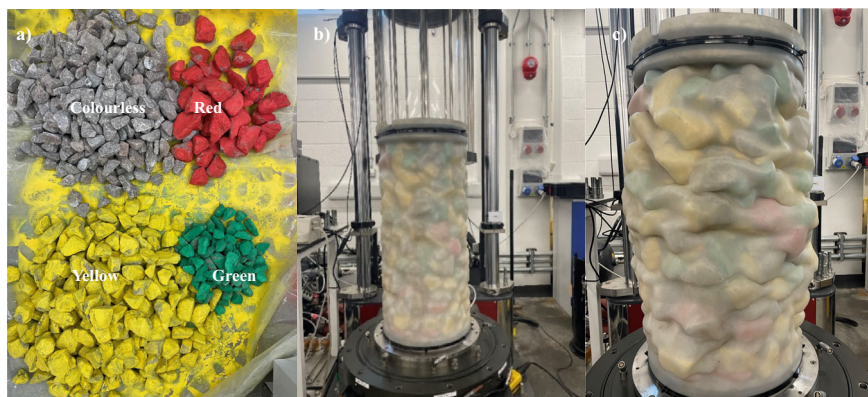
Fig. 2 a Ballast sample used in test 3 (63 mm > Red > 50 mm > Yellow > 40 mm < Colourless < 31.5 mm < Green < 22.4 mm. b Test 3 sample before the test. c Test 3 sample after the test
