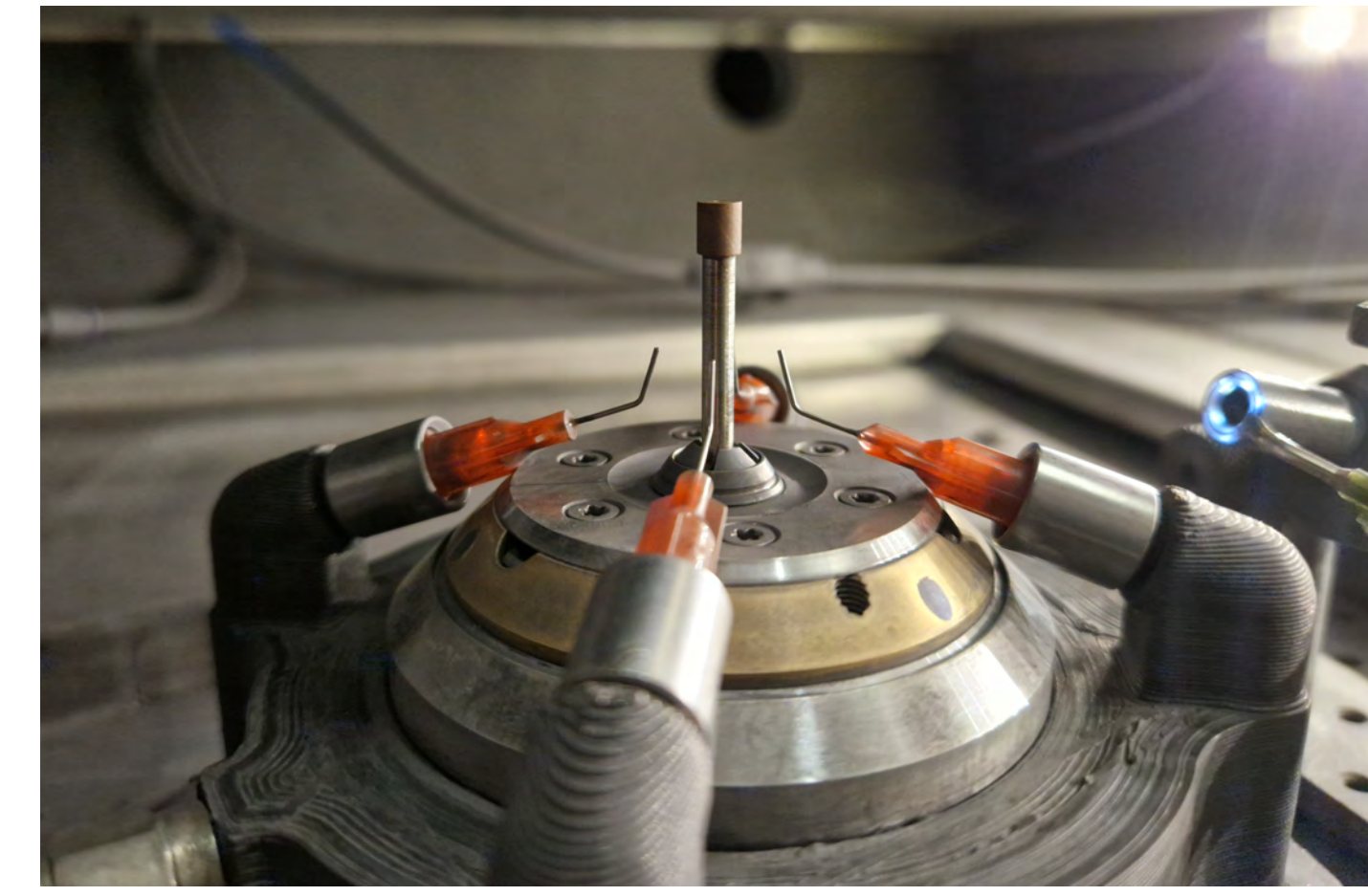
An image of the tool in Loxham machine spindle.
