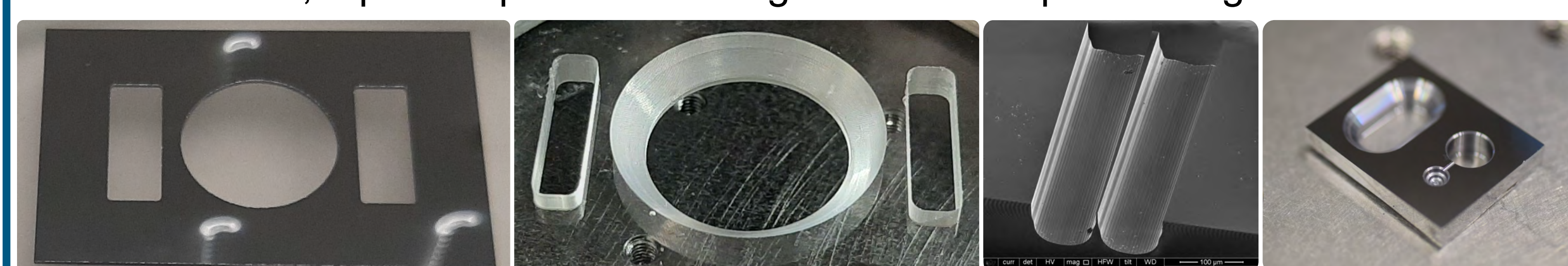
Examples of milling work in silicon, silica, and lithium niobate.
