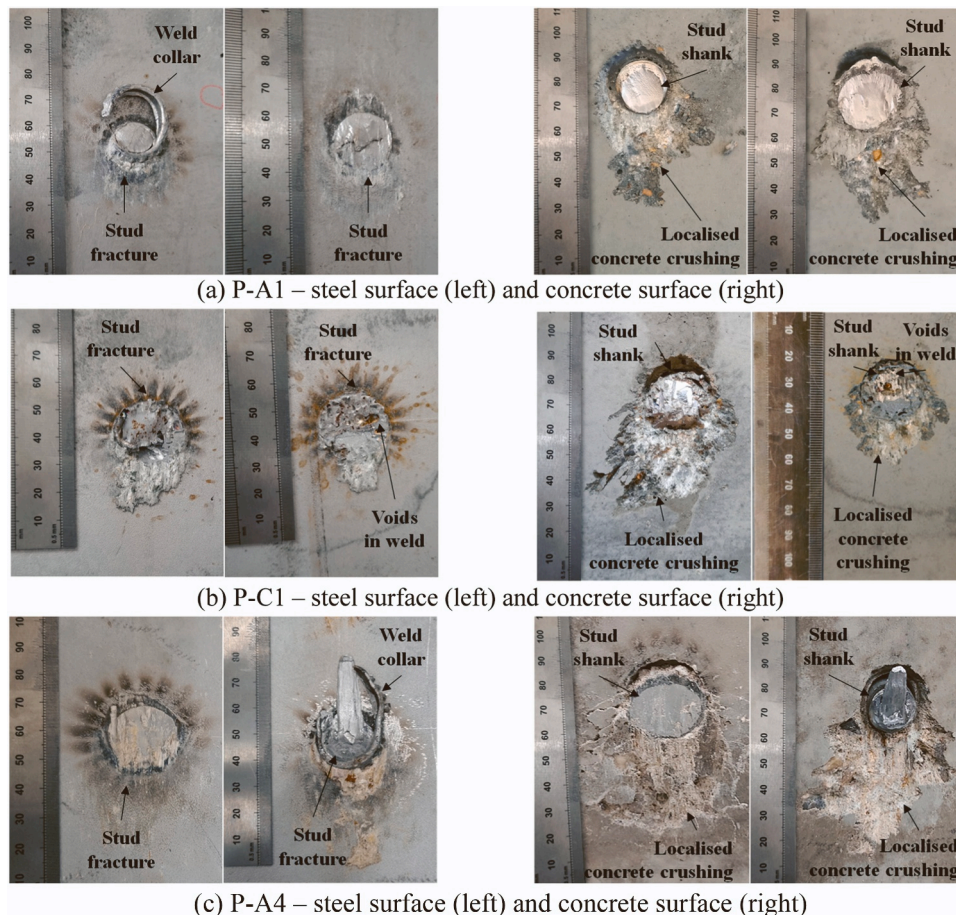
Fig. 16. Photographs of steel and concrete damage after push-out tests.
