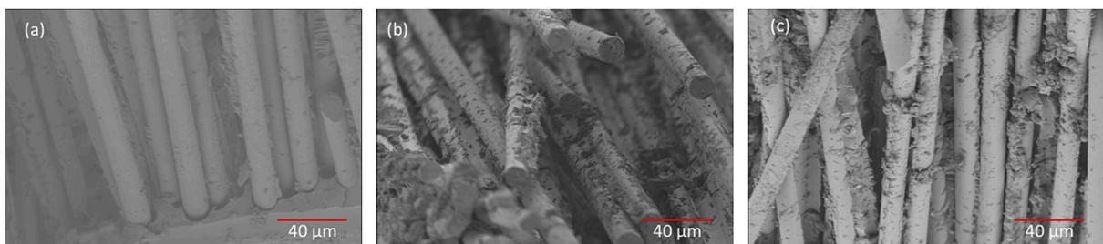
Fig. 7. SEM micrographs of the fracture surfaces after the tensile test a) glass-carbon/epoxy without coating, b) 1 wt% GNP coated glass-carbon/epoxy and c) 5 wt% GNP coated glass-carbon/epoxy composites.
