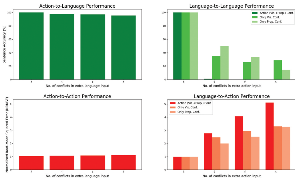
Figure 7. Model performance on the test set wrt. no. of conflicts introduced in the extra input. For action-to-language and language-to-language (the top row), we show the predicted sentence accuracies. For language-to-action and action-to-action, we show the normalized root-mean-squared error (NRMSE) for predicted joint values. The modality in which the conflicts are introduced is given in the x-axis. For each signal, we add extra conflicting inputs either in the action or language input. When the conflict is introduced in action, we also test having the conflict only in the vision and only in the proprioception submodality - in this case, the other submodality has the matching input.
