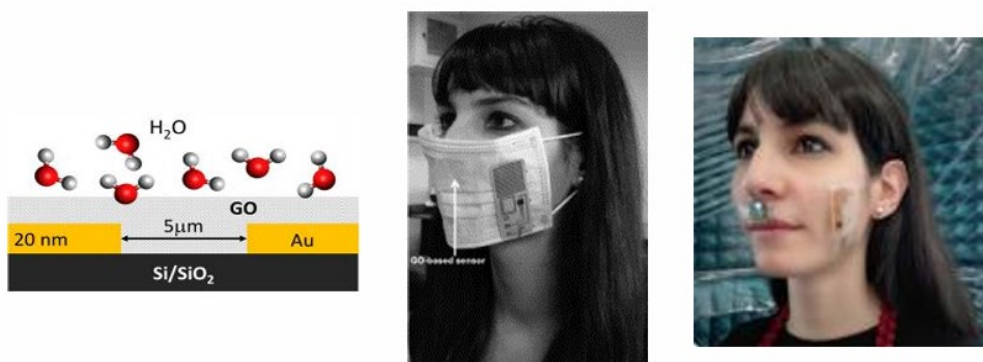
Figure 23 Schematic diagram, prototype and actual deployment of graphene oxide humidity sensor[49][50].
