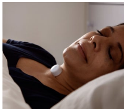
Figure 24 ACURABLE AcuPebble wireless acoustic based respiration sensor mounted on the neck of a subject[52].
