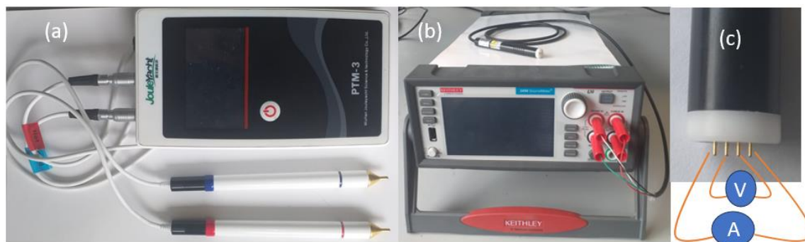
Figure 2.13. Room Temperature Transport Properties Measurements (a) Portable ThermoElectric Meter for Seebeck coefficient measurements, (b) Keithley Source meter-2450 with four-point probe, (c) magnified 4-probe indicating current source on outer probes while inner two-probe for voltage.
