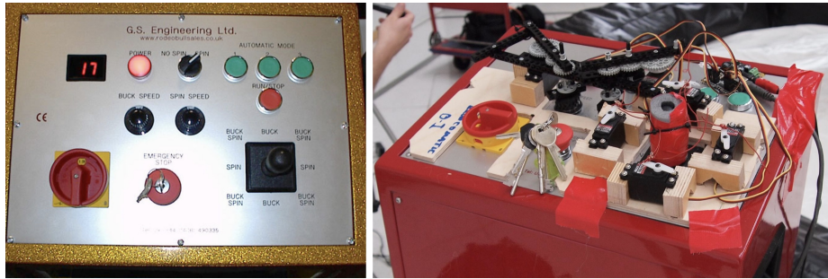
Fig. 2. Left: The Broncomatic control interface. Right: Using Lego Mindstorm technology to safely manipulate the controls.
