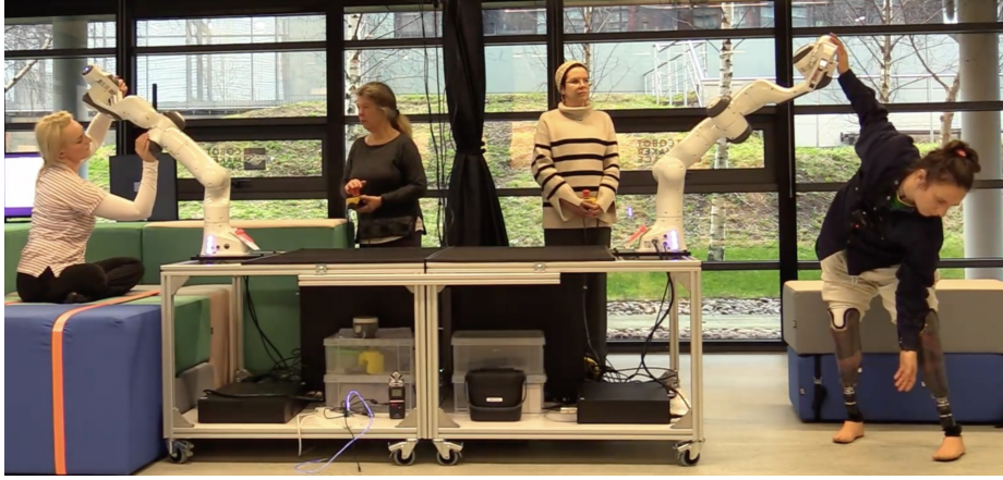
Fig. 4. Dancers with different disabilities dancing in harmony with a pair of Franka robot arms. To ensure safety, each robot is independently monitored and equipped with an emergency stop button for immediate cessation of operations if needed.
