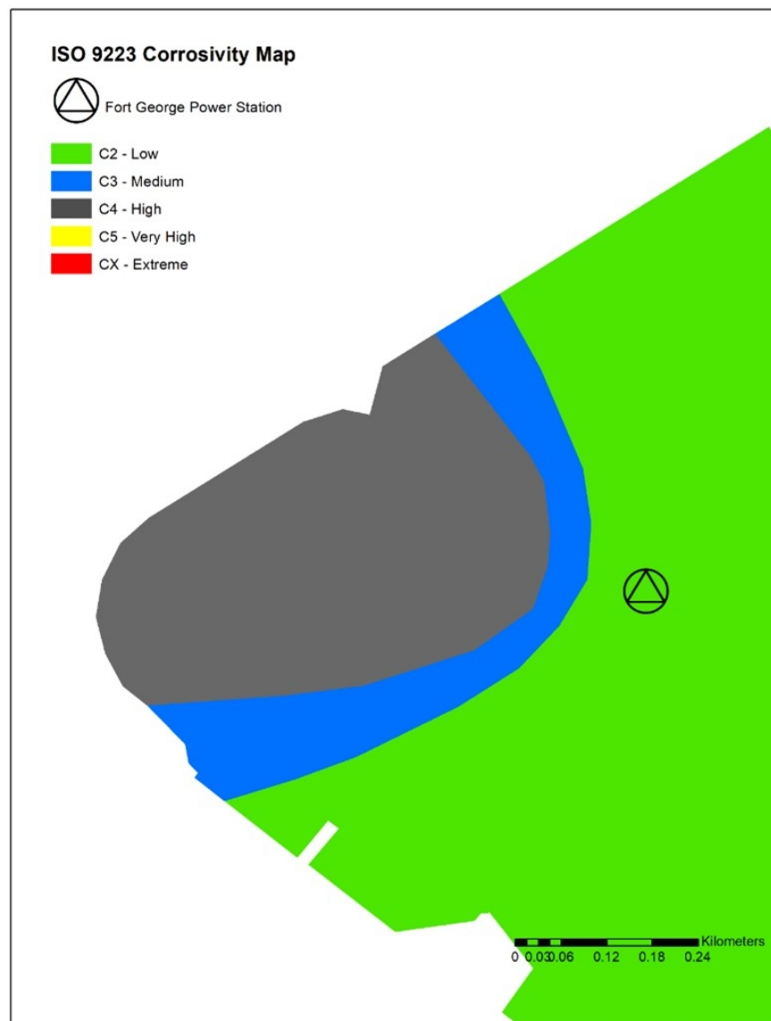
Figure 6. Corrosion map generated as a vector data model, showing the most aggressive area in Port-Louis around 200 m downwind of Fort George Power Station.
