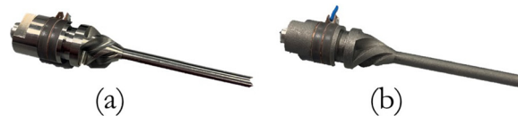
FIG. 3. (Color online) Ultrasonic needles with (a) MA and (b) DMLS Ti-6Al-4V components.
