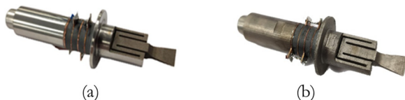
FIG. 4. (Color online) Ultrasonic planar twice folded bone cutting devices with (a) MA and (b) DMLS Ti-6Al-4V components.
