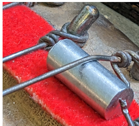
FIG. 7. (Color online) Cylinder used to lift the string to decouple it from the soundboard.
