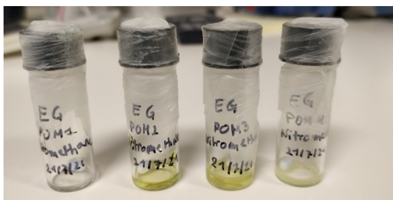
FIGURE 5.4: Pictures of \text{H}_3\text{PW}_{12}\text{O}_{40} , \text{H}_3\text{PMo}_{12}\text{O}_{40} , \text{Na}_3\text{PMo}_{12}\text{O}_{40} , (\text{NH}_4)_3\text{PMo}_{12}\text{O}_{40} 10 mg/mL solutions in nitromethane.
