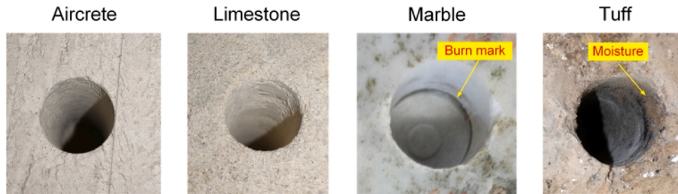
Fig. 9. UAD drill holes in aircrete, limestone, marble and tuff.
