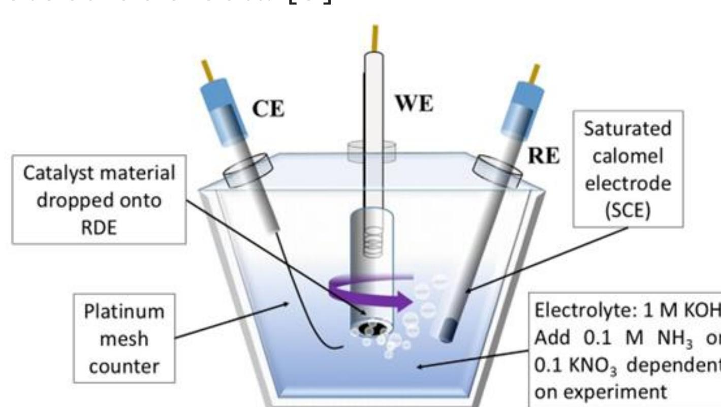
These experiments investigate the electrochemical oxidation of ammonia and reduction of nitrate.
