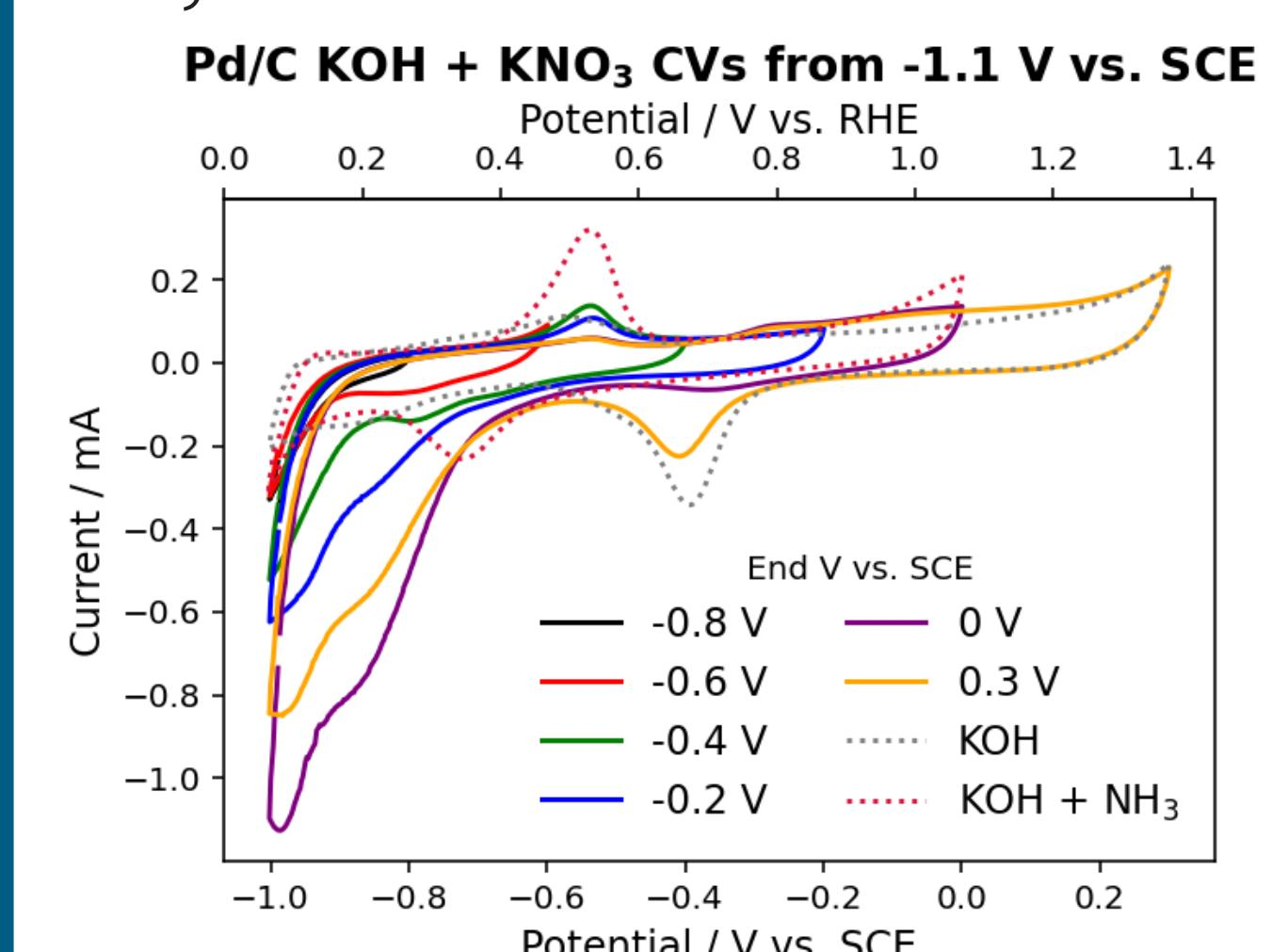
Nitrate reduction can form ammonia as seen by ammonia oxidation peak which could be due to palladium nitride formation.
