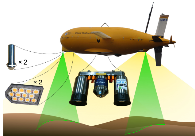
FIGURE 6. BioCam setup on ALR. The main housing containing the cameras and electronics is mounted centrally. Sheet lasers and LED strobes are mounted one each at the front and the back of the vehicle.
