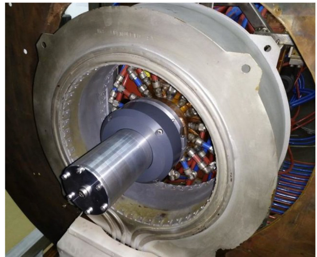
Fig. 9. The SX3 AF-MPD thruster of the IRS within its large applied-field coil [43].
