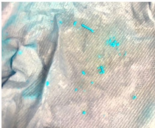
Figure 7.2: Image showing HKUST-1 removed from the Repligen device hollow fibre filter lumen after flushing with ethanol post-experiment.
