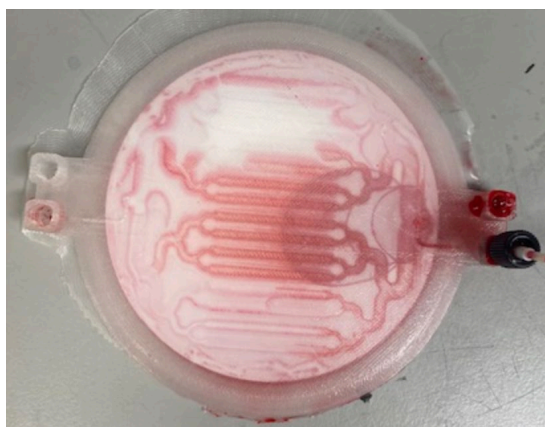
Figure 6.12: The third test print with a pipe diameter of 2.5 mm fabricated using the PPP technique after food dye had been infused, showing how dye infused through the \frac{1}{4} -28" inlet on the right passed through the membrane and exited the let next to it when it should have passed through the channel system to the let on the left side of the device. It also shows how the dye bled throughout the device below the membrane and did not follow the channel system.
