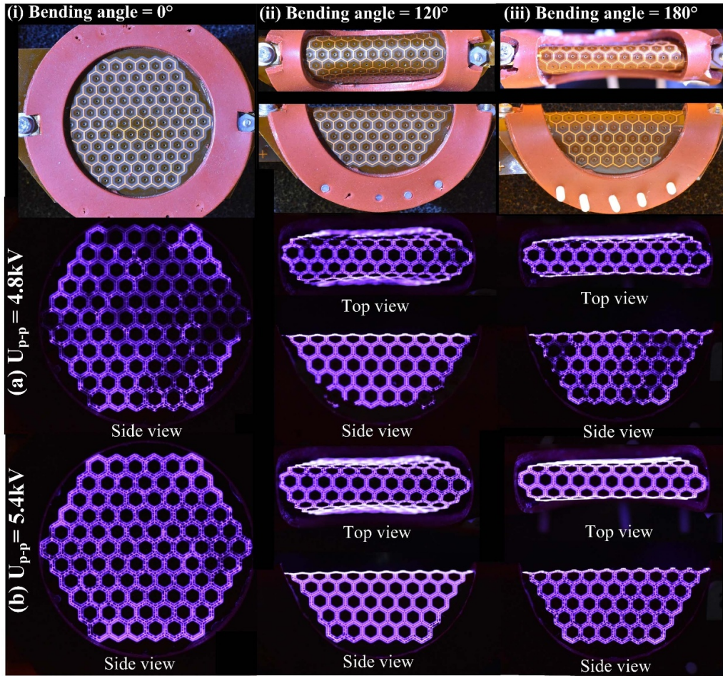
Figure 3. Discharge images under different curved electrode conditions when the applied voltage was fixed at (a) U_{p-p} = 4.8 kV and (b) U_{p-p} = 5.4 kV (exposure time 1 s, ISO 3200, f/6.3).
