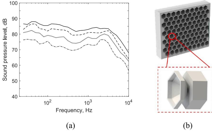
**Fig. 4.** (a) Typical one-third octave noise spectra at 25 m from a TGV-Duplex train running at different speeds;  $\cdots$  200 km/h;  $\cdots\cdots$  250 km/h;  $-\cdot-\cdot-$  300 km/h;  $---$  350 km/h [49]. (b) Acoustic EH device proposed by Wang et al. [47].
