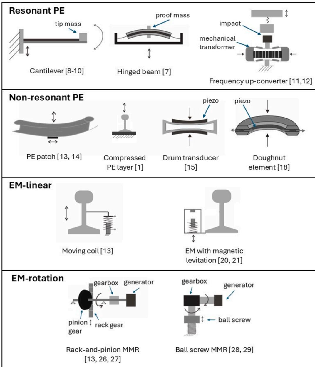
Fig. 1. Illustrative diagrams of vibration energy harvesting devices.
