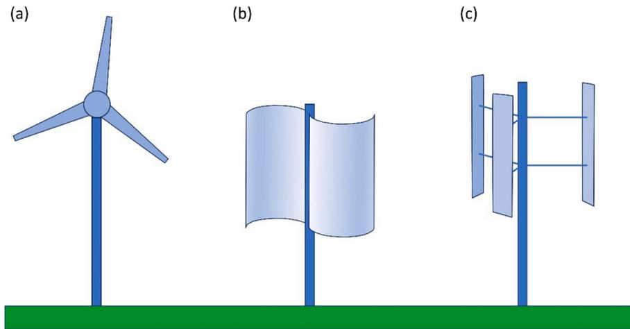
Fig. 3. The three main types of wind turbine: (a) HAWT, (b) Savonius VAWT, and (c) Darrieus VAWT.
